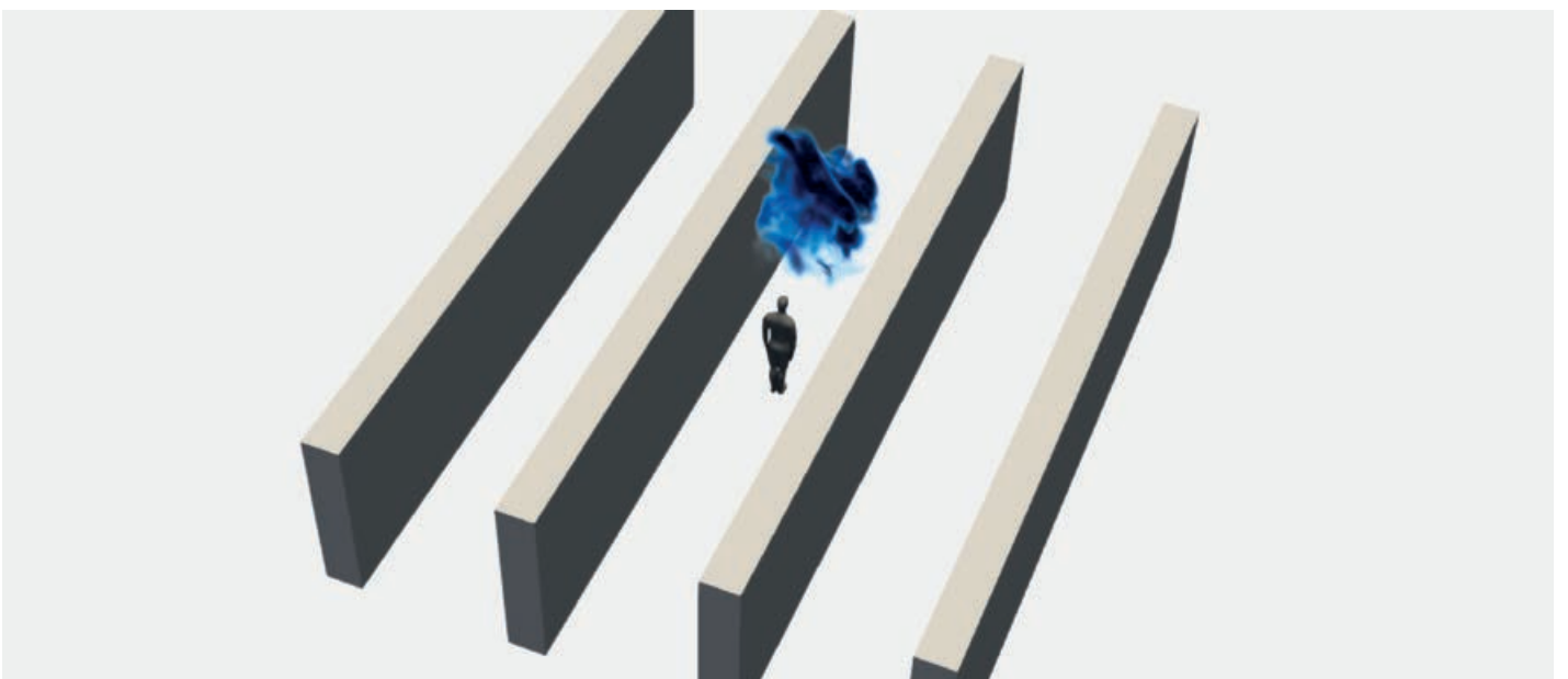
▼ Figure 4. Researchers from four Finnish research organizations modelled a situation in which a person coughs down a shelf-restricted corridor typical of grocery stores (picture by Petteri Peltonen / Aalto University) (Aalto University, 2020).
