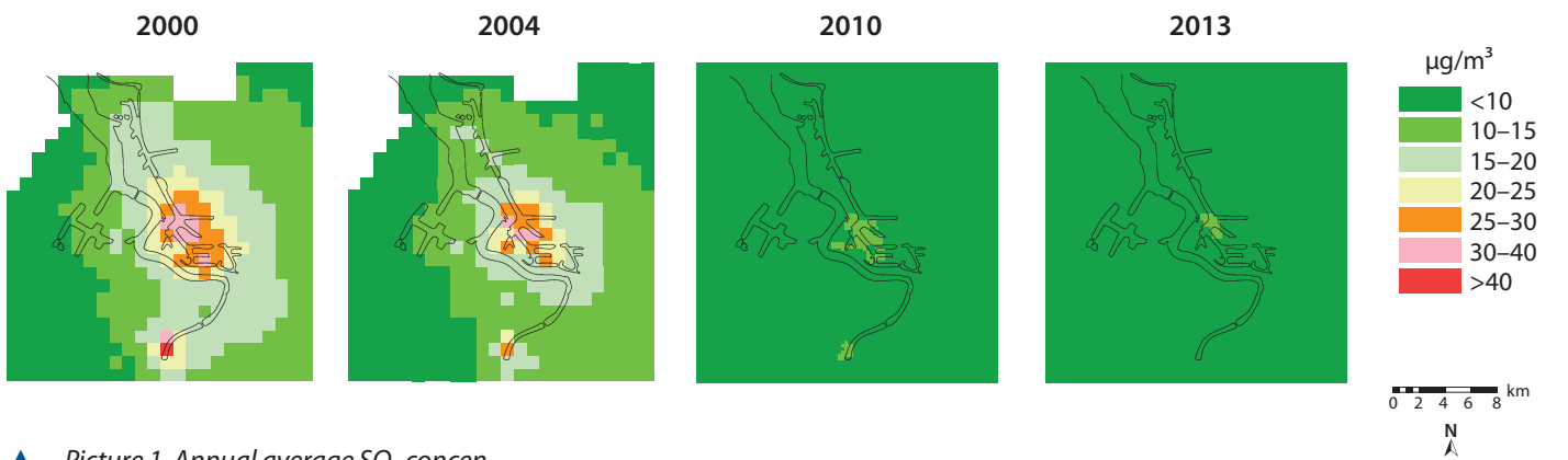
▲ Picture 1. Annual average SO 2 concentration in the port of Antwerp in 2000, 2004, 2010 and 2013. The level of SO 2 concentration in the port and city declined so dramatically that the map colour key had to be changed from 2010 onwards (on the right) to allow for SO 2 levels below 10 µg/m 3 . In order to allow a meaningful comparison, the 2010 and 2013 maps from the Flemish Environment Company were redrawn (above) according to the 2000 and 2004 map key for this publication.
