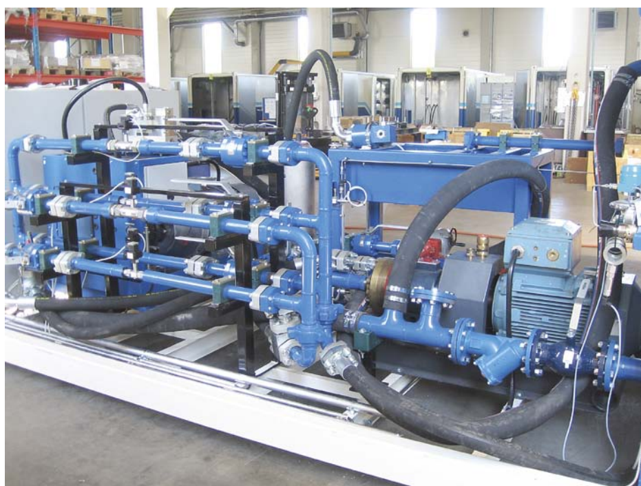
▲ The WQ laboratory testing device used to simulate oil well features
