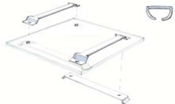
Paper machine maintenance hatch , easily manufactured
